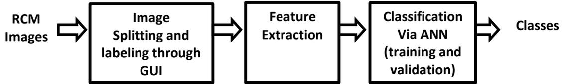
**Figure 3.** The main steps of the classification algorithm.
