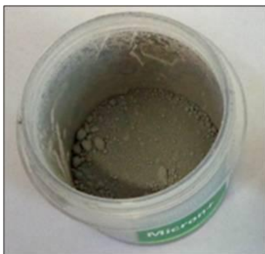
Figure 1. Photo of the 250 nm ElementSix nanodiamond powder.
