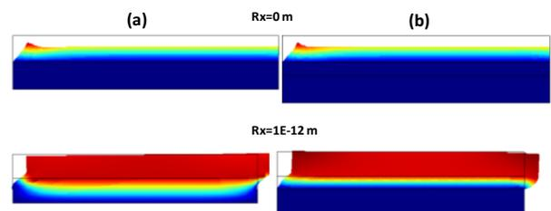
Fig.4.: Coatings displaced by applying loads on (a) Ti/NCD and (b) Ti/TiC/NCD. The 2D FEM deformations refer to  $R_x = 0$  m and  $R_x = 10^{-12}$  m.
