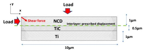
Fig.2: Mechanical 2D FEM modelling of NCD/TiC/Ti multilayered structure.
