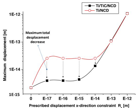
Fig.3: Maximum total displacement versus  $R_x$  for Ti/TiC/NCD e Ti/NCD multilayered structures.
