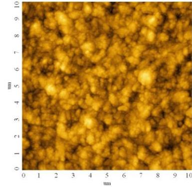
Fig.1: AFM topography image of NCD coating grown by MWPECVD.
