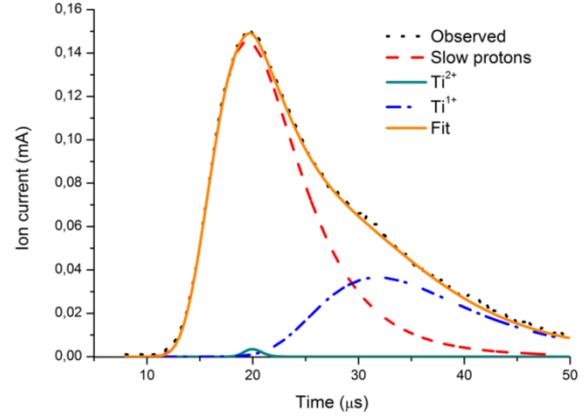
**Figure 4.** Deconvolution of the TOF signal obtained in free expansion at a 0.6 GW/cm<sup>2</sup> laser irradiance.
