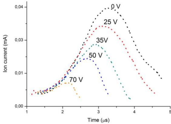
**Figure 3.** TOF proton currents for different stopping voltages applied to EB at 5.1 GW/cm<sup>2</sup> in free expansion.
