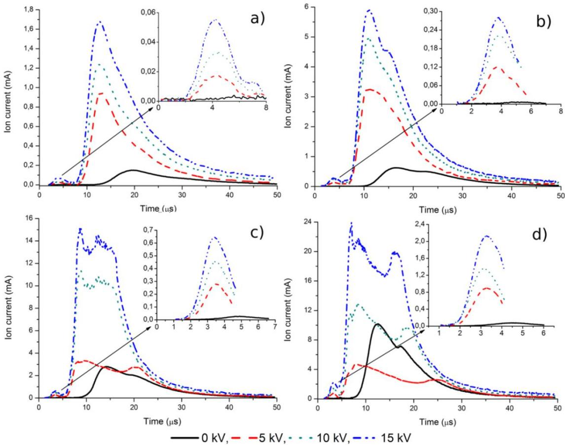
**Figure 2.** Ion currents recorded on FC by a digital oscilloscope at 0.6 (a), 1.3 (b), 2.5 (c) and 5.1 (d)  $\text{GW}/\text{cm}^2$ , for different accelerating voltages.
