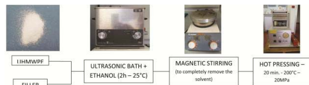
Figure 1 – Flow sheet of the preparation steps of the filled polymer.
