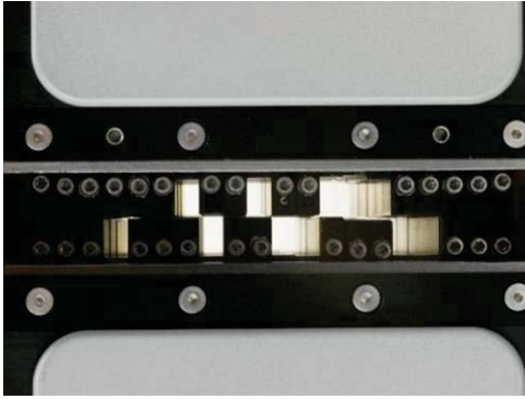
Fig.1 MIMiC view from patient toward target of the gantry
