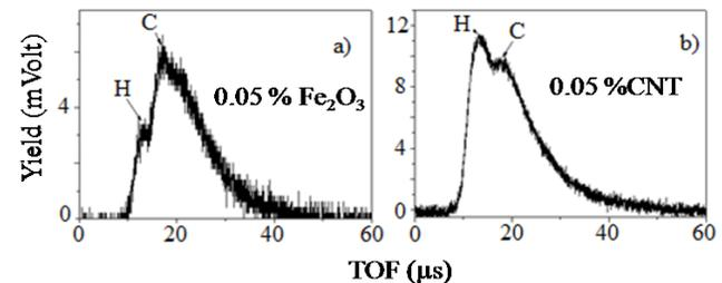
Fig. 5: Two IC experimental spectra detected at a laser pulse energy of 150 mJ and in backward configuration for UHMWPE+Fe<sub>2</sub>O<sub>3</sub> (a) and UHMWPE+CNT (b) thin films, at 0.05% doping concentration.
