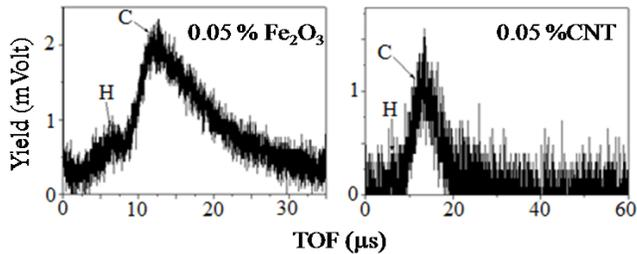
Fig. 7: Two IC experimental spectra detected at a laser pulse energy of 150 mJ and in forward configuration for UHMWPE+Fe<sub>2</sub>O<sub>3</sub> (a) and UHMWPE+CNT (b) thin films, at 0.05% doping concentration.
