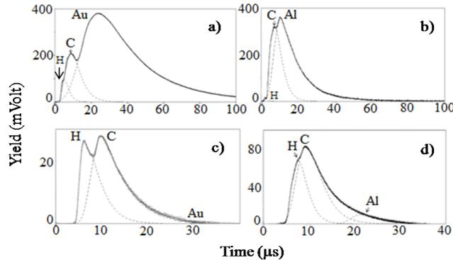
**Fig. 2:** Four typical IC1-TOF spectra obtained irradiating, from the metal side, the 500  $\text{\AA}$  Au thin film covering 3.5  $\mu\text{m}$  mylar film (a), the 0.1  $\mu\text{m}$  Al covering 3.5  $\mu\text{m}$  mylar film (b), and, from the polymer side, the 100  $\mu\text{m}$  mylar covered with 500  $\text{\AA}$  Au film (c) and 3.5  $\mu\text{m}$  mylar covered by 0.1  $\mu\text{m}$  Al (d), and detecting the ion emission in backward direction.
