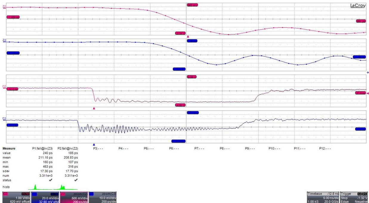
Fig. 7. Waveforms of the input signal (Z2) and of the response (Z3) at 10 ns time scale and at 200ps time scale. In this case the resistor is inserted inside the central electrode.
