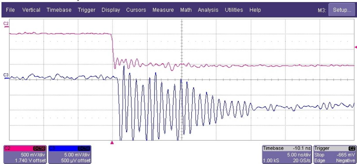
Fig. 6. Waveforms of the input signal (C2) and of the response (C3) at 10 ns time scale with the load after the divisor electrode.
