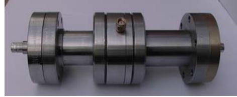
Fig. 5. Photo of the transmission line containing the capacitor divisor.
