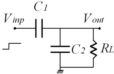
Fig. 2. Schematic diagram of a capacitive voltage divisor:  $C_1$  is the capacitance of divisor electrode and external conductor,  $C_2$  is the capacitance of the internal conductor and the divisor electrode.
