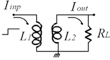
Fig. 1. Schematic diagram of an inductive current divisor:  $L_1$  is primary inductance,  $L_2$  is the secondary inductance.
