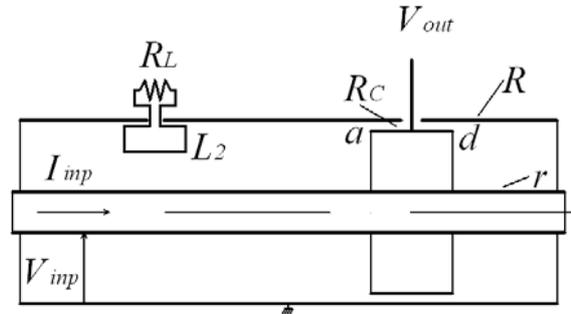
Fig. 3. Sketch of the transmission line, inductor divisor (loop closed on a very little  $R_L$ ) and capacitive divisor (capacitor closed on very large load) geometry.
