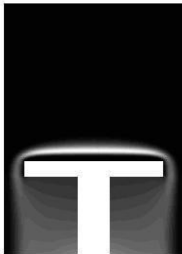
Fig. 1. Layer of particles during AlN growth in a vertical reactor, predicted by the computations.
