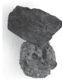
Fig. 5: SiS.18.33.9, slag with charcoal.
