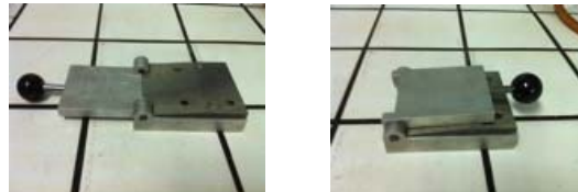
Figure 1: Device for bending resistance tests
