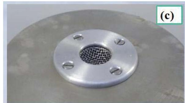
Figure 2: Photos of the extraction hole without a grid (a), with a plane grid (b) and with a curved grid (c).
