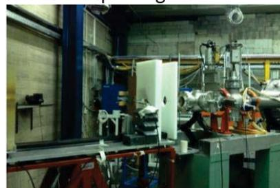
Fig. 4: Setup in the experimental area for the 62 MeV proton irradiation at INFN Laboratori Nazionali del Sud (Catania, Italy).
