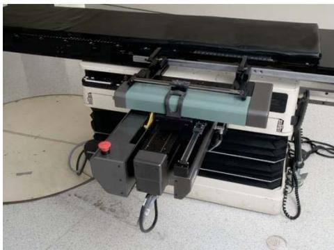
Fig.2 AutoCrane mounted on linac couch
