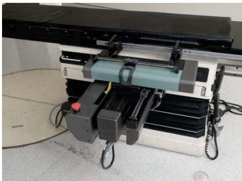
Fig.2 AutoCrane mounted on linac couch
