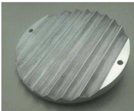
Fig. 5: Faraday cup collector  $90^\circ$ .
